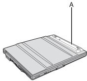
At the time of purchase, the stylus (included) is not attached to the stylus holder (A). The tether prevents the stylus from falling accidentally. It can be attached to the stylus holder.
